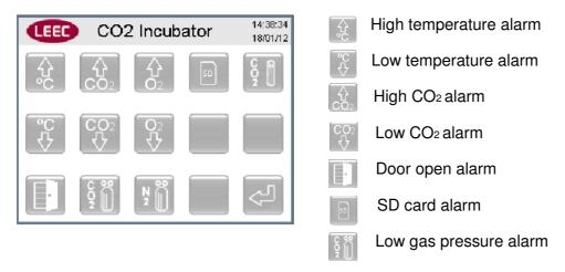
In an alarm condition an audible buzzer sounds and the alarm icon changes to red. Press this red alarm icon and the alarm status screen will show the corresponding alarm will in red. For instance this shows high temperature alarm condition: Pressing this will mute the alarm. The alarm is now acknowledged and the icons show this by changing to yellow: The icons remain yellow for as long as the incubator is in an alarm condition. This process is the same for all alarms.
