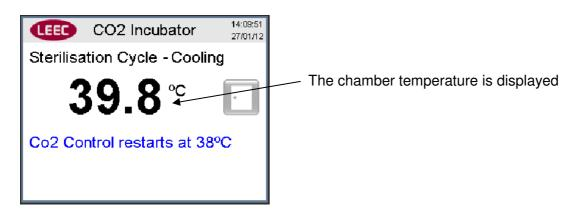
The cooling phase ends once the temperature falls below 38.0 °C
