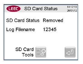
Insert the SD card into the slot to the right of the controller (label side closest to controller).
