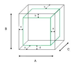
A, B, C = Internal dimensions a = distance from left and right wall = 70mm b = distance from top = 70mm c = distance from front and back wall = 70mm d = distance from base = 70mm
