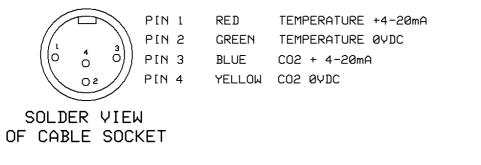
The temperature signal is scaled as: 4mA = 0 °C; 20mA = 250 °C
